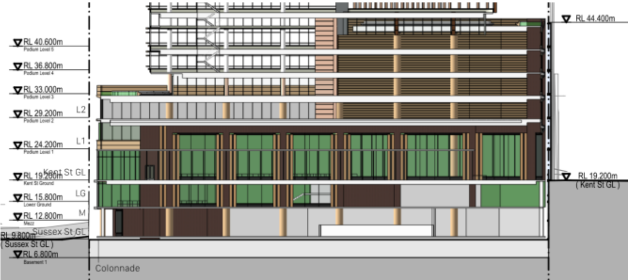
Figure 4 - Architectural East-West section
